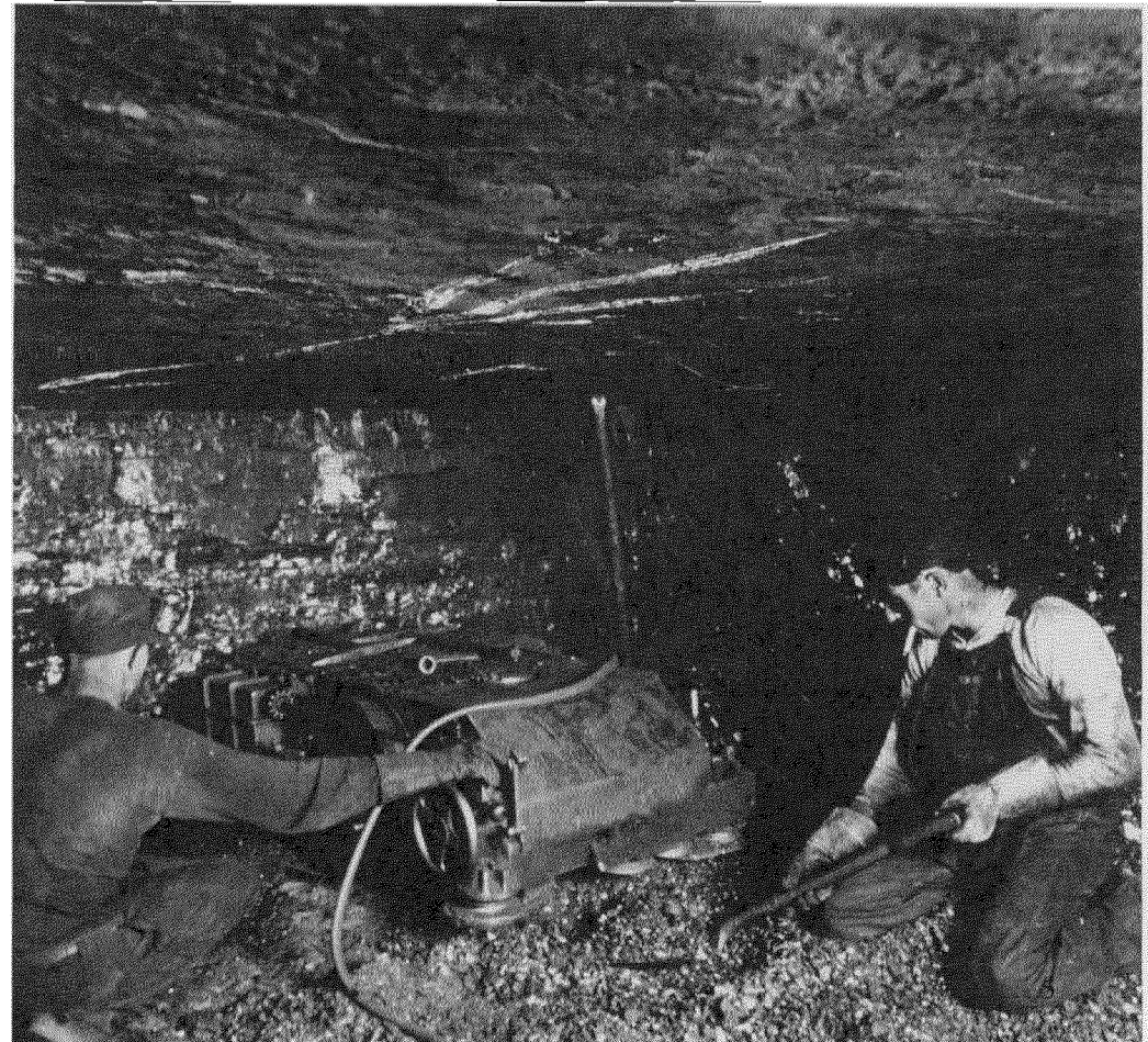
Mine power supplied a big portion of KU's load when this electric coal cutting machine was in use in 1922.
